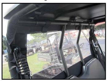
1. Lay the Dust Panel over the roll cage of the vehicle making sure the straps are on the outside of the roll cage. Secure the top straps first. If some straps interfere with the hardtop mounting configuration, omit the attachment of those straps.
